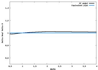
Comparison with the equivalent pipe method
